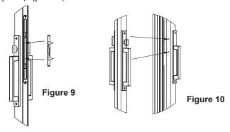
13. Using the dimples as a guide, install the keeper to the panel with the dummy handle using the (4) #8 x 1-1/4" pan head screws. Adjust the keeper up or down until the latch engages properly, (Figure 11).
