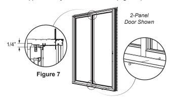
10. Install the provided plastic roller adjustment hole plugs when adjustment is complete.
