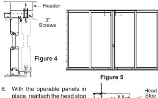
With the operable panels in place, reattach the head stop by replacing the 1" Flat Head screws that you removed in step 2 (Figure 6).
